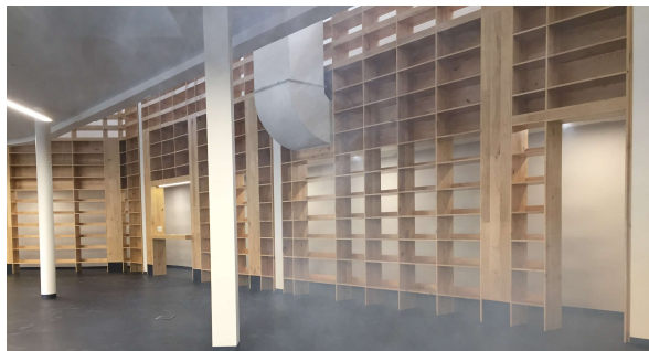
Smoke testing – to visualise air movement
