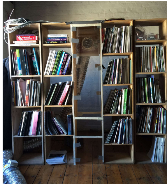
Library bookshelves test setup front view. Transparent ventilation diffuser.
