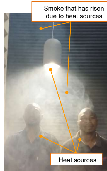
Smoke for demonstration rising at “heat sources”.
