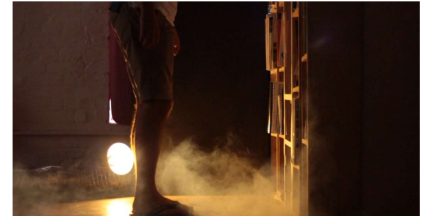
2. Person (heat source) steps into the air flow.
